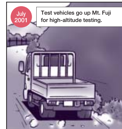
10 Another challenging issue was to demonstrate engine performance at high temperatures. The engine must be tuned so that coolant water temperature does not rise too far, reducing engine power, even when the gas pedal is floored while the truck is climbing a steep slope.
