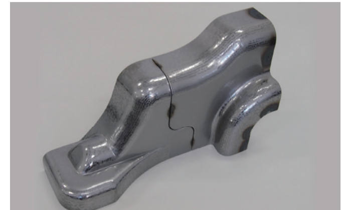
Bronze medal-winning automobile plating assignment work Produced from a single steel sheet according to drawn instructions within the working time (7 hours)
