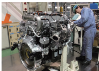
Engine being reassembled
