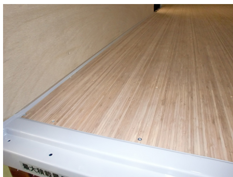
A vehicle utilizing bamboo flooring material
